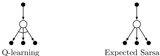
Figure 6.4: The backup diagrams for Q-learning and Expected Sarsa.
