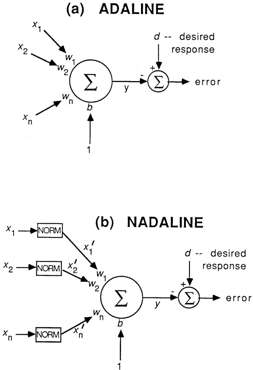
Figure 1. The primary difference between the classic ADALINE and the NADALINE is a local normalization of the input signals.
