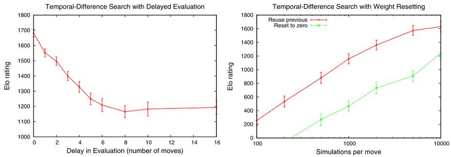
(a) TD search with 10,000 simulations/move. The results of the latest search are only used after a  $k$  move delay. (b) Comparison of TD search when the weights are reset to zero at the start of each search, to when the weights are reused from the previous search.
