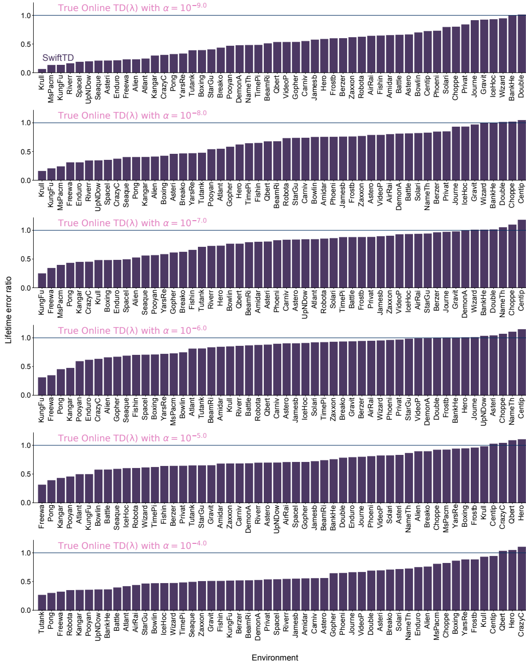
Figure 7.4: SwiftTD with fixed hyperparameters compared to True Online TD( \lambda ) with different values of the step-size parameter. For all values of \alpha , SwiftTD achieved a lower lifetime error than True Online TD( \lambda ) on a majority of the games.
